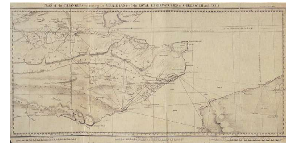
Image of 'Plan of the triangles' connecting the meridian of Greenwich and Paris
